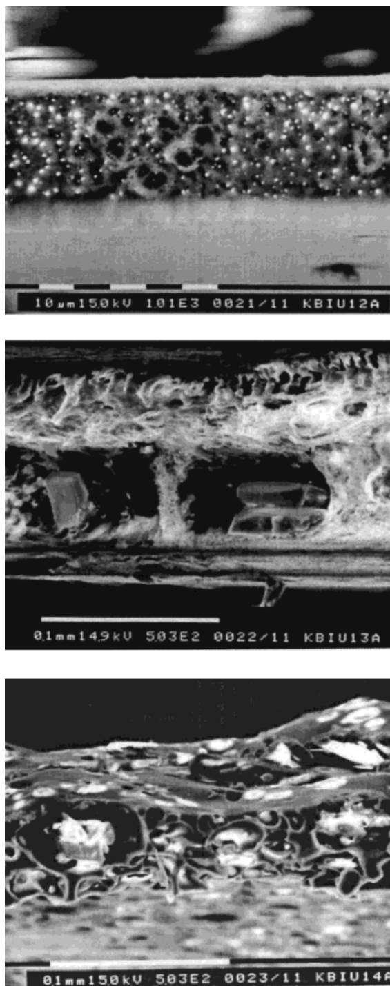
Figure 3 Scanning electron micrographs of cross sections of membranes with progesterone; membranes are prepared by vacuuming (top), immersion precipitation (middle), and vapor exposure (bottom).
